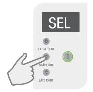
The display shows SEL (Select). Select the temperature by pressing the buttons. 1, 2 or 3 is shown in the display.
