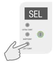
The display shows SEL (Select). Select the temperature by pressing the buttons. 1, 2 or 3 is shown in the display.
